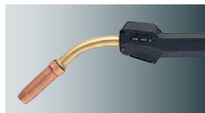
SB 307 G mixed gas: 280 A 60% duty cycle CO 2 : 300 A 60% duty cycle
