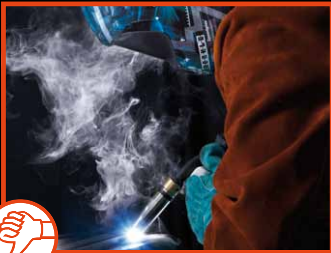
Standard welding torch: strong fume production!
